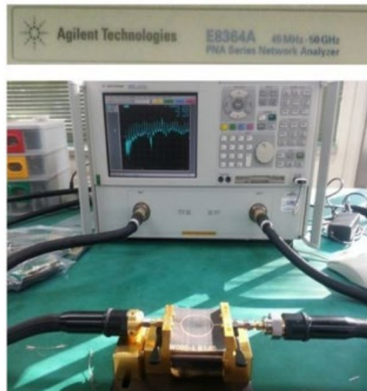
Agilent E8364A PNA Network Analyzer and Universal test fixture 3830 K (by ANRITSU) were used for ring resonator testing.
