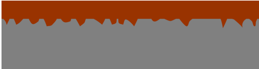
Figure 2 – Illustration of copper laminated to PTFE surface.
