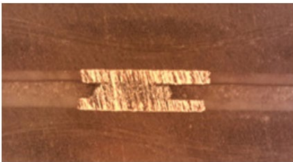
fastRise™ prepreg between subassemblies w/copper paste
