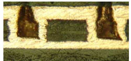
6 mil microvia laser ablated by Micron Technology, Inc. Preliminary data suggests that the optimal lasing conditions are a combination of CO 2 and UV lasers.
