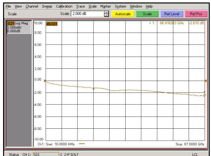
Microstrip insertion loss of EZ-IO-0050 (2.61 dB/in at 67 GHz) using Southwest Connectors (12.45 mil trace width, 0.5 oz HVLP)
